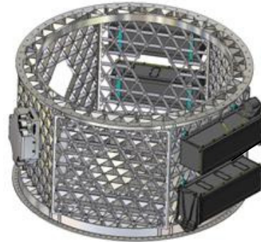
RSA Structure with example Payloads
